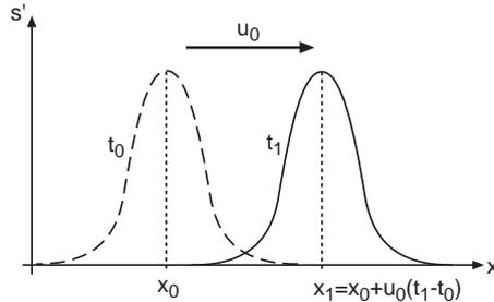
Figure 6.2: propagation of an entropy wave in 1D
