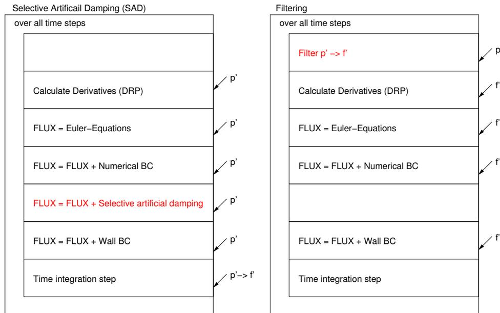
Figure 10.3: Selective artificial damping and filtering implementations in comparison ( $f'$  denotes the filtered,  $p'$  the original field)
