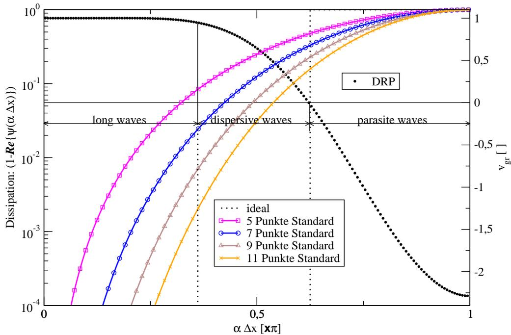
Figure 10.6: Different standard filters and the DRP depending on  $\alpha\Delta x$
