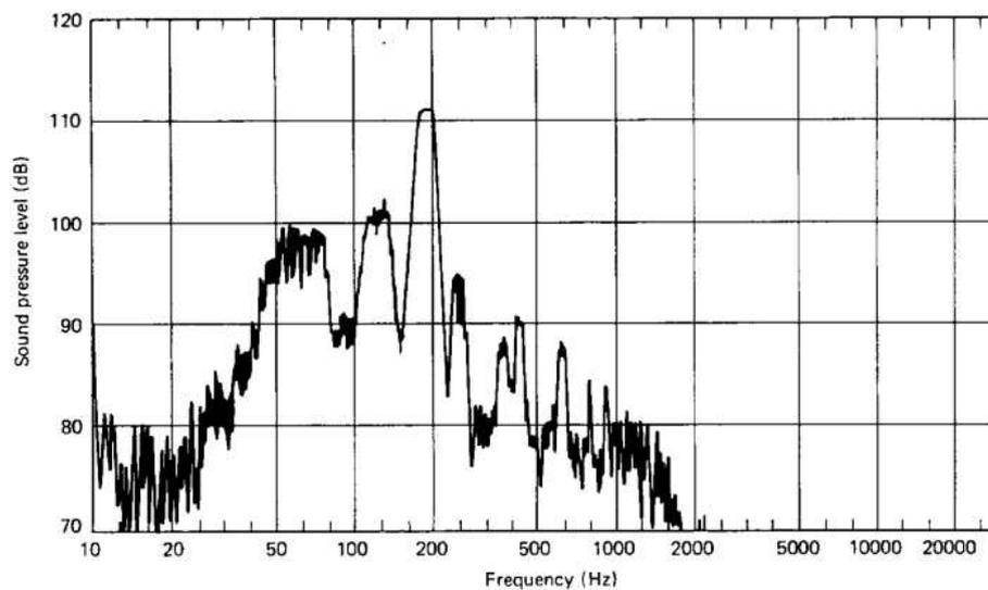
Figure A.1: Sound Spectrum of an Air-Compressor
