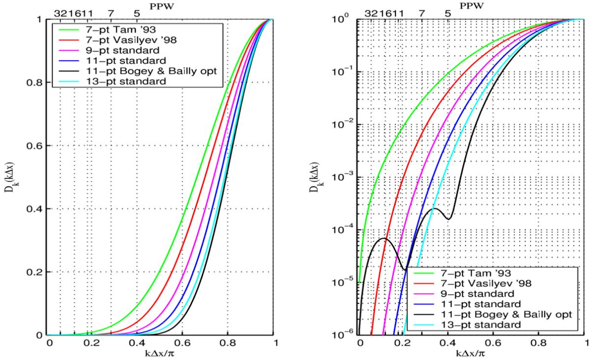
Figure 9.1: Filtering characteristics of different filter stencils
