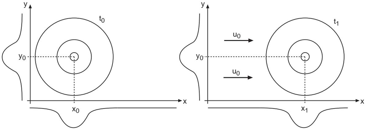
Figure 6.3: propagation of an entropy wave in 2D
