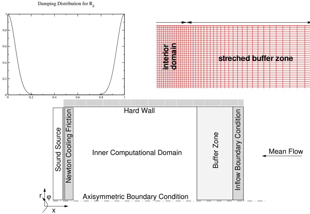
Figure 12.1: Damping distribution and stretched axisymmetric grid
