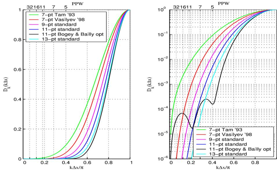
Figure 10.2: Filtering characteristics of different filter stencils
