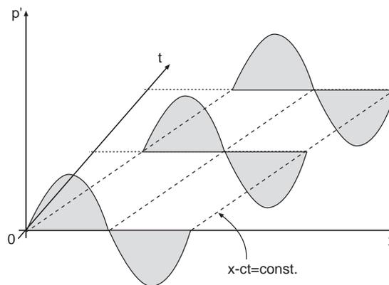
Figure 1.10: Characteristic of a plane wave
