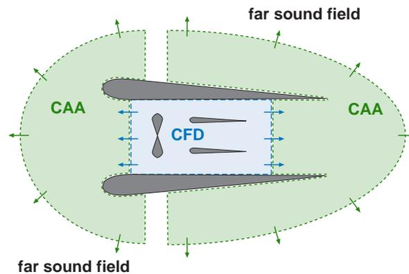
Figure 1.9: Zonal approach to compute engine noise
